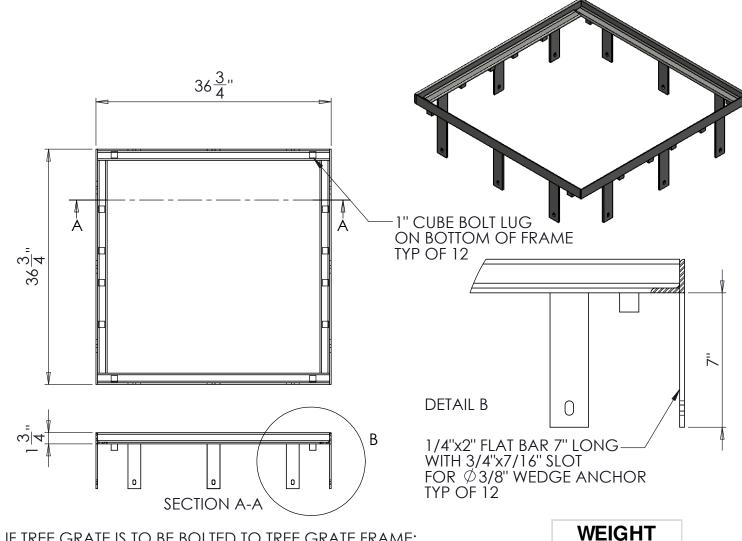
IF TREE GRATE IS TO BE BOLTED TO TREE GRATE FRAME: ORDER SBF ID#D00BD "BOLT DOWN KIT". EACH KIT CONTAINS:
